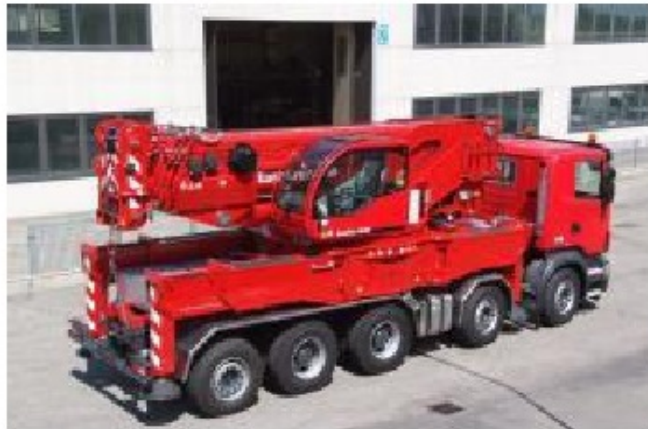
Eurogru Amici: Crane 200.23 capacity 200 tons
