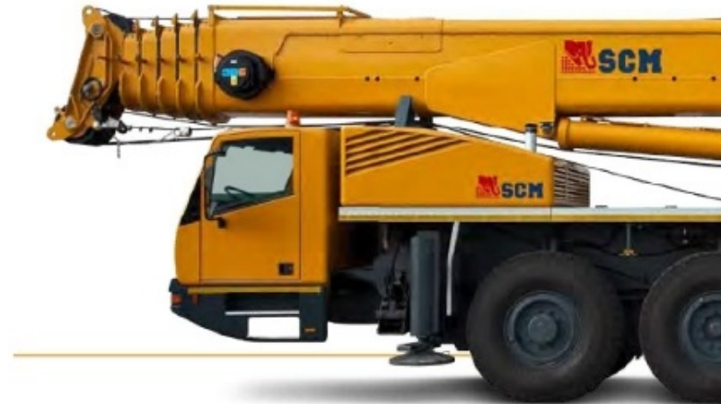
SCM: Crane SA4100 capacity 100 tons
